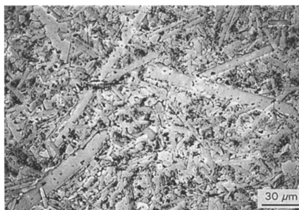
Figure 1 Scanning electron micrograph of the SiC surface etched for 13 min by a boiling Murakami solution of 3 g KOH and 30 g \text{K}_3[\text{Fe}(\text{CN})_6] in 60 ml \text{H}_2\text{O} .
